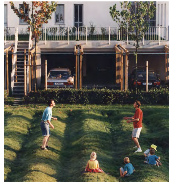
Figure 7.15: Potsdam, Germany, this example of a courtyard space within a block of housing contains parking at ground floor level, with residents' private deck areas above and a communal garden area in the centre
