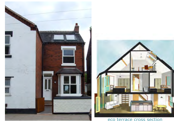
Figure 2.21: Eco terrace, Chesterton - the existing housing stock will need to be upgraded as part of adapting for climate change. This example demonstrates how Victorian terraced houses can be retrofitted to raise their environmental performance to meet today's requirements
