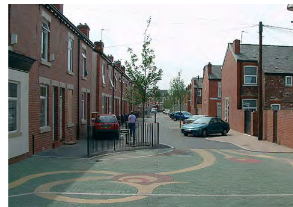
Figure 7.13: Changes of surface material, combined with a narrowing of the street space and tree planting, provide visual interest and help to keep traffic speeds low in this example of a homezone
