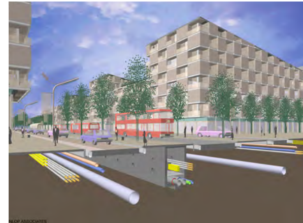
Figure 2.2: Elephant & Castle, London - one of the first zero carbon growth town centre redevelopment proposals, for a significant area at the heart of Elephant & Castle. It will incorporate an area-based Combined Heat and Power system, water supply and data services, all managed by a Multi-Utility Services Company, which has been established by Southwark Council
