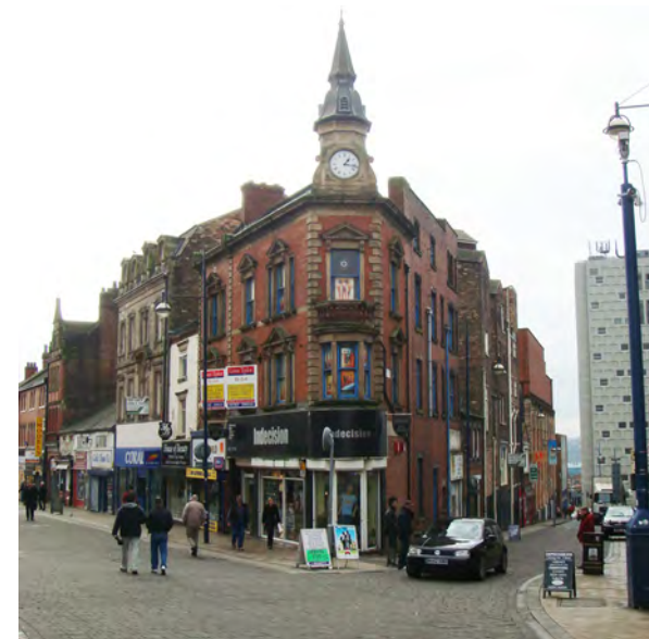
Figure 4.6: A corner plot on Brunswick Street and Piccadilly addressed by the built form. Here the corner is chamfered with a small clock turret. The facade is ornate, with a small scale, using typical local materials of red brick and buff sandstone dressings
