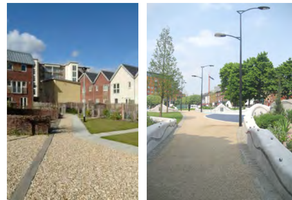
Figure 11.4: Examples of high quality footways following desire lines and with clear sight lines to provide easy and direct routes and encourage walking
