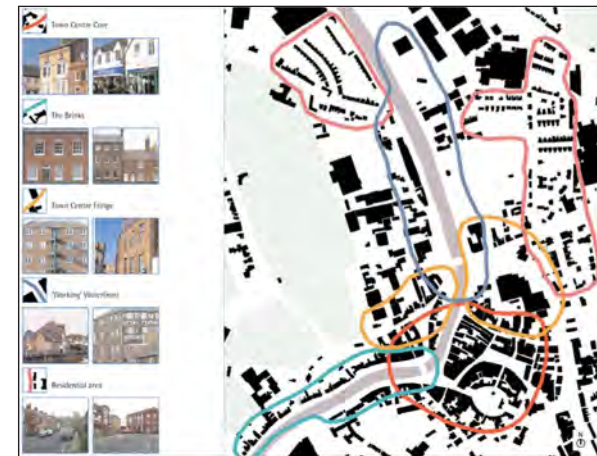
Figure 3.7: A figure ground diagram shows the built form in black and spaces left as white, as here. This can help to identify different patterns of development, here highlighting the character of the built form
